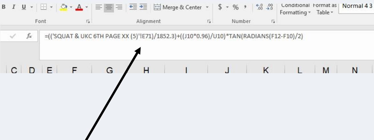
Calculation formula applied on cell for wheel over calculation on each leg.
