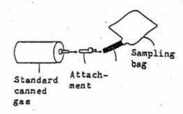
into the smaping bag. When the sampling bag is filled with the span gas, stop pressing the nozzle to the attachment, bend the rubber tube and nip it by a pinch cock. Next, pull off the attachment from the rubber tube.
